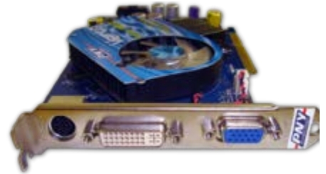
Graphics Card Model: PNY, nVidia 6600GT Gold colored edge in the right-rear of the photo is slotted on the motherboard. External ports are then provided, as shown in the foreground. public domain image
