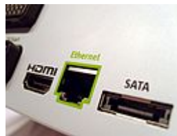
eSata Port — By Declan Jewell from Stevenston, Scotland (Sky HD Box) [CC-BY-2.0] , via Wikimedia Commons
