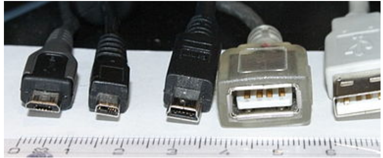
Different USB connectors. From left to right: male Micro USB B-Type, proprietary (not USB), male Mini USB (5-pin) B-type, female A-type, male A-type, male B-type. Shown with a centimeter ruler. Female A-type connector (4th from left) is "upside down" to show the pins. By Viljo Viitanen (Own work) [Public domain], via Wikimedia Commons
