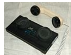
Acoustic coupler modem (very old ~300 bits/s)— public domain image
